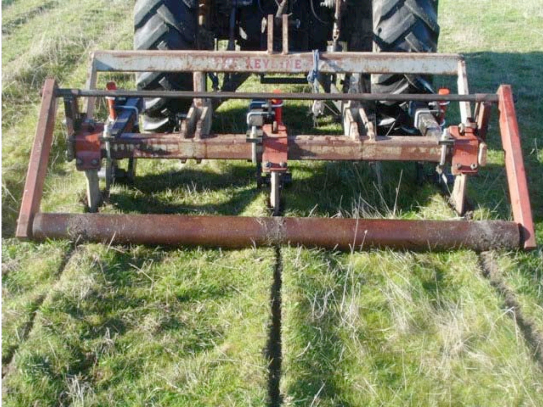
Figure 3. Yeomans Keyline plow in operation. Note the minimal disturbance to the soil surface.
