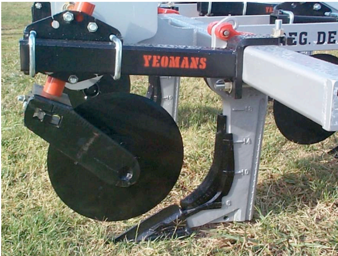
Figure 2. Yeomans Keyline plow shank with attached coulters.
